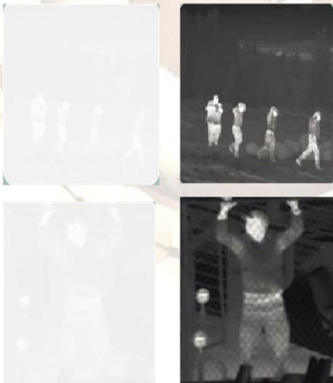
Fig. 4 Few snapshots of using thermal camera in foggy weather
